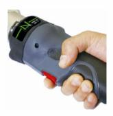
5. Press the release button to retract the piston
