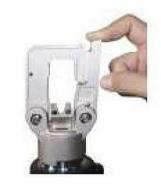
4. Slide the dies into the open head. Make sure the dies are matching and seated correctly.
