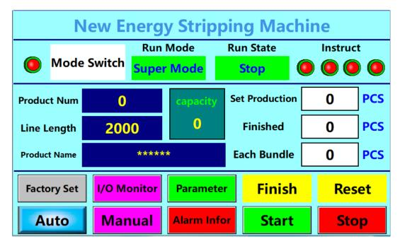
**Mode Switch:** Stripping mode, three-layer mode, short-line mode, super mode (ultra-short wire length mode) can be switched freely, each mode has specific operation instructions; (Available to equip with inkjet code device, marking device, slitting and partial stripping function)
