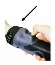
Pull back the lactch to open the head. The head will spring open
