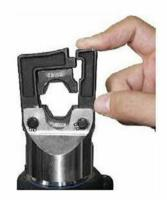
Slide the dies into the open head. Make sure the dies are matching and seated correctly.
