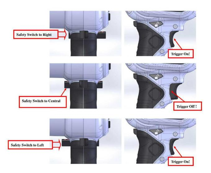
4. When the tool is sitting idly or once you are finished with it, put the tool switch in the central position.
